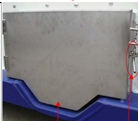
Bottom cabinet cover Takigen snap lock
